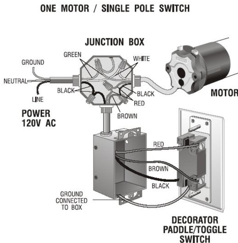
**NOTE:** Your switch may not exactly represent the unit depicted in the above diagram. If not, connect the **BLACK** (AC Power HOT) to the **BLACK** screw of the switch. Connect the **BROWN** (Motor Direction #1) to one of the brass-tone screws, and connect the **RED** (Motor Direction #2) to the remaining brass-tone screw. Reverse the **BROWN/BLACK** and **RED** connections if the motor is installed on the **LEFT** side of your door opening.
