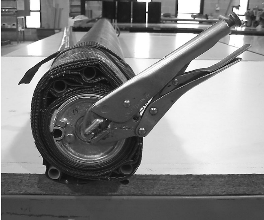
Photo #4 (Setting Spring Pre-Load)
